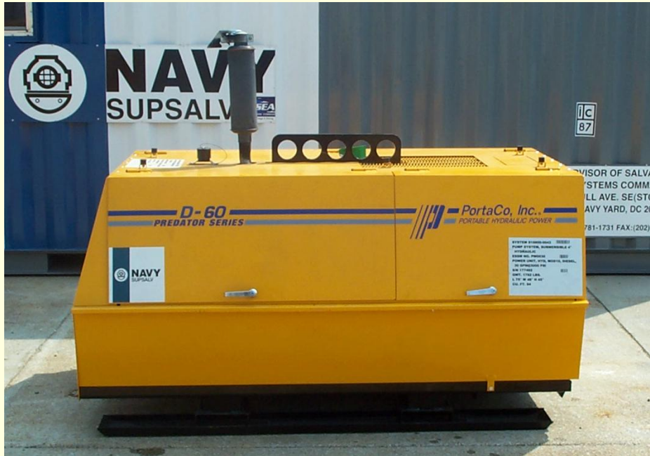
Mod 10 Hydraulic Power Unit PW0030
