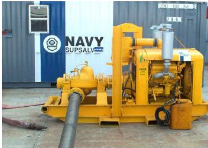
2 1/2-Inch Jetting Pumping System using PU0229
