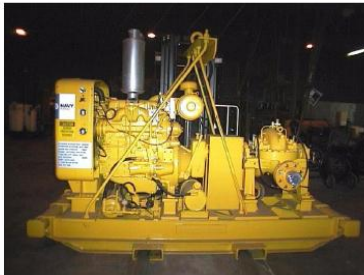
2 1/2-Inch Jetting Pumping System using PU0228/PU0230
