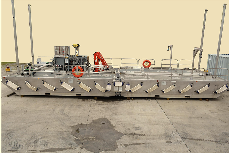
48' x 16' x 4' Modular Working Platform BA0005 (with Modular Oil Bladder Transfer System VA2290 components)
