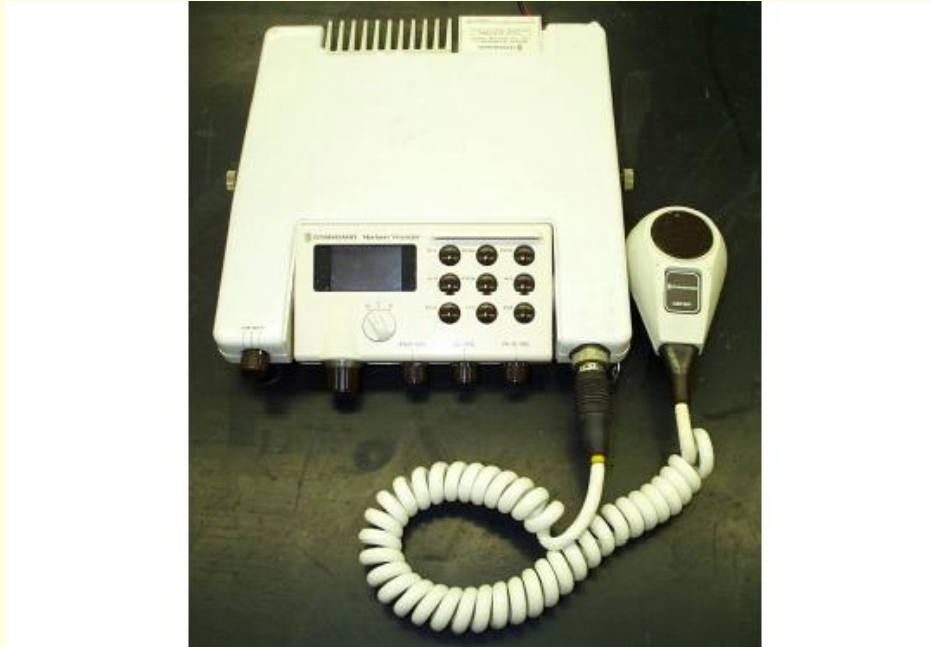
76-Channel Voyager Marine Mobile VHF Radio RA1830
