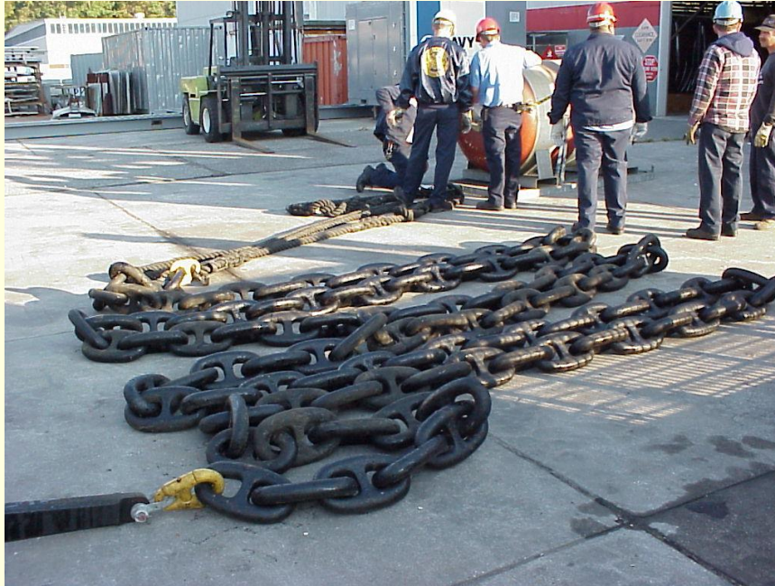
2 1/4" x 90' Cast Steel Chain CH0002
