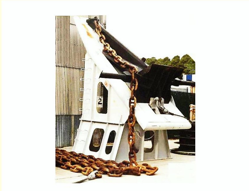
4-Point Mooring System Anchor Billboard AN0080
