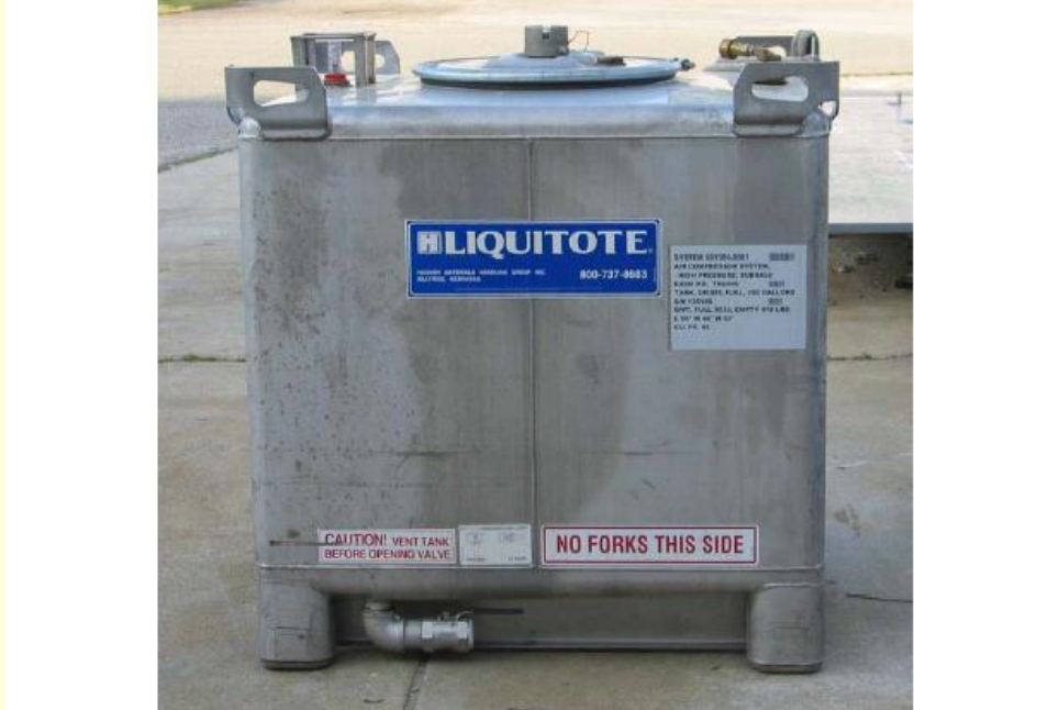
350-Gallon Diesel Fuel Tank TK0040
