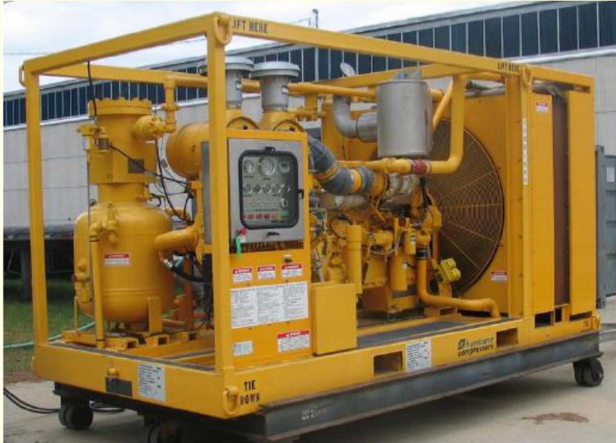
Submarine Salvage Air Compressor AC0245
